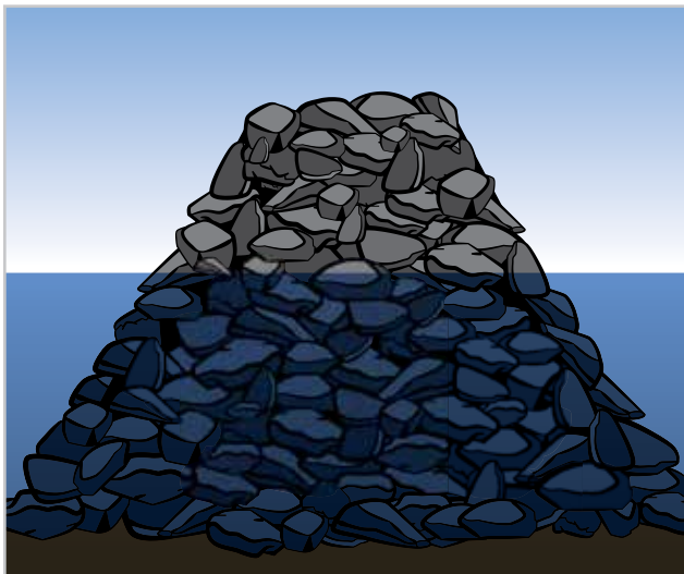
Rock jetties have a wide base on the ocean floor.
